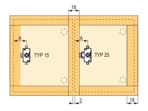
• an example of the use of locks type 750.15 and 750.25 (the same distance between the lock and the edge of both full overlay and half overlay cabinet doors)
