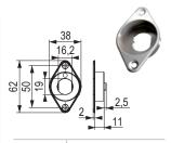
fixing element for mounting into wood
