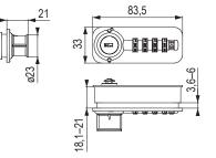
Drawing of hole in board 18.1-21 mm for locks types 57, 58, 59.
